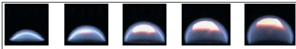
Figure 6: Laminar jet fire of C_2H_4 at microgravity conditions. (Zhang et al , 2015b)
