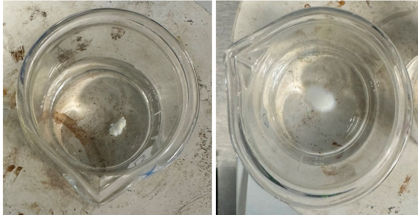
Figure 29. Aqueous test environment before (left) and after (right) the swelling test.
