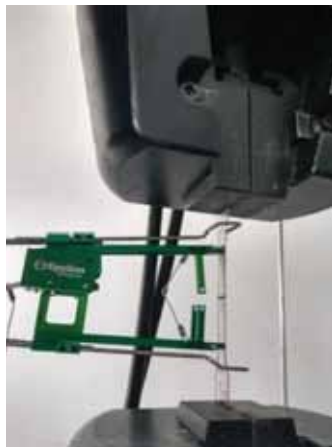
Figure 4. Tensile Test being performed with Epsilon Extensometer.
