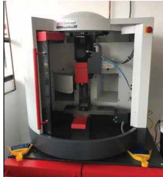
Figure 9. CNC Milling machine EMCO concept MILL 55 taken from (Belmont Galvez, 2018)
