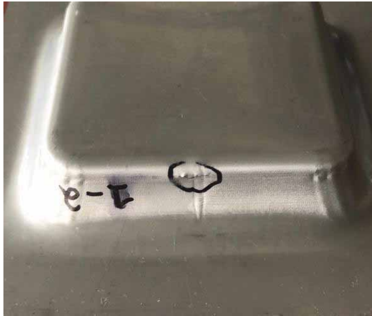
Figure 64. Detail Image featuring the fracture of a VWA part
