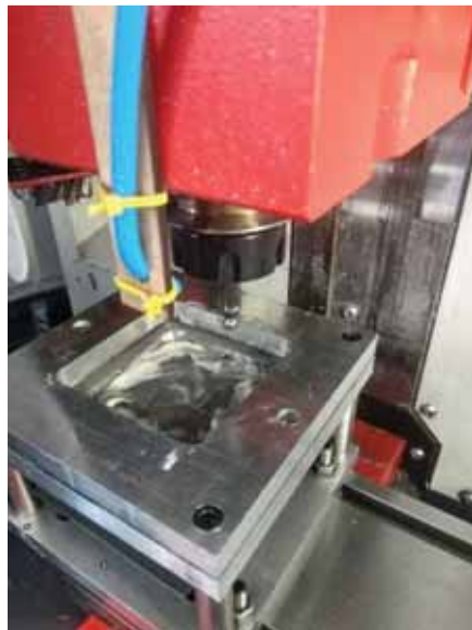
Figure 1. SPIF tool, blank holder, and lubricated blank
