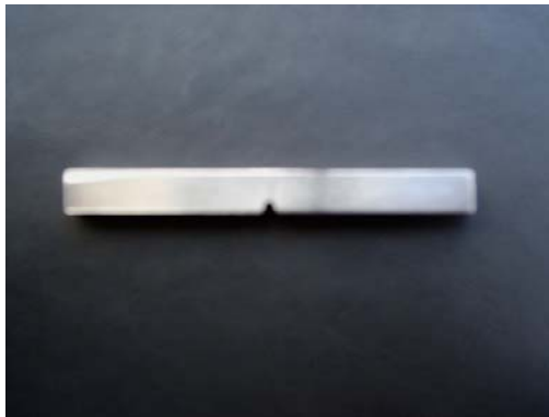
Fig. 2.6. Impact test standard sample.
