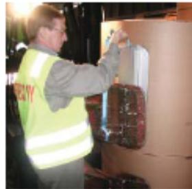
Due to its thin design, the Test Pad adapts to changing roll diameters.
