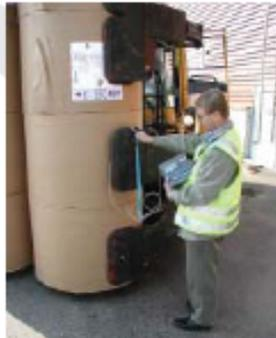
Clamping forces are equally easy to measure from a wide angle of paper roll clamps.
