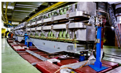
(c) The Proton Synchrotron (PS) pipe where hadrons are accelerated with superconducting magnets and reach an energy of 25 GeV
