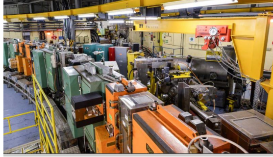
(b) Proton Synchrotron Booster(PSB). Third stage of accelerating ions. Energy reached of 1.4 GeV
