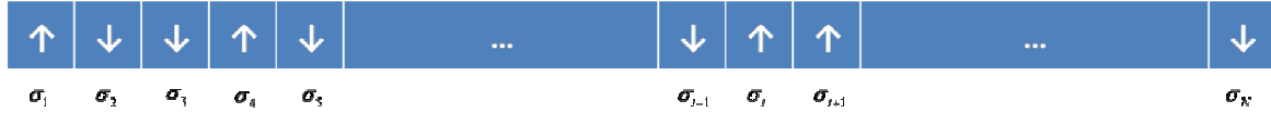
Figure 15. A system of atoms represented by their magnetic moment in a lattice which is parallel or anti-parallel to an external magnetic field.
