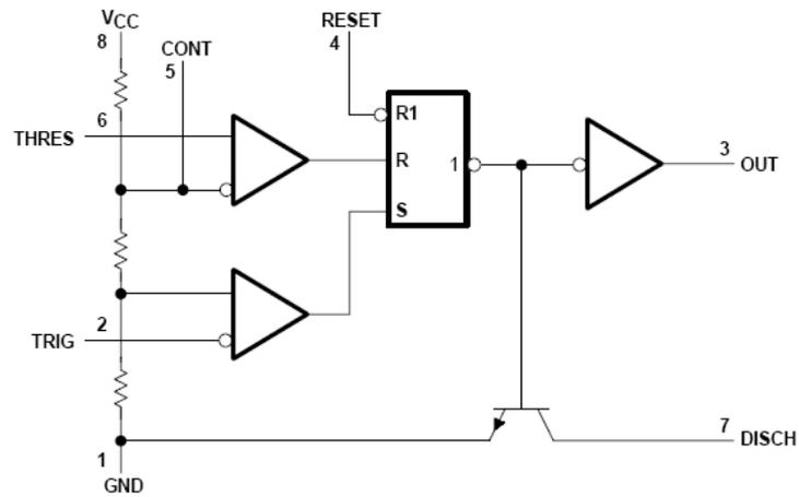
Pin numbers shown are for the D, JG, P, PS, and PW packages.
