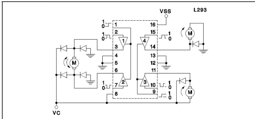
Note: Output diodes are internal in L293D.
