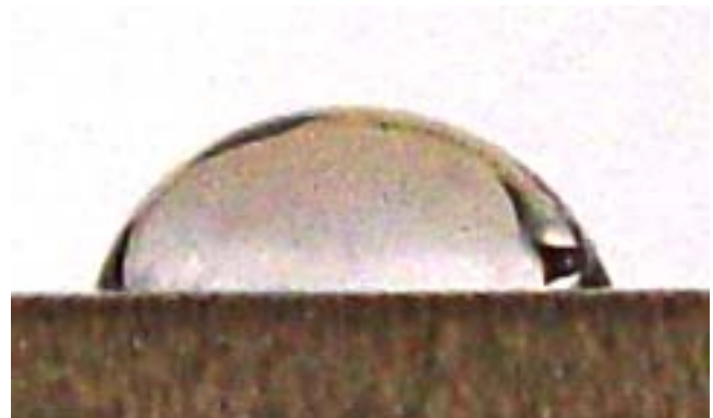
Figure (2) The contact angle of a solution of water-ethanol-propilenglycol.
