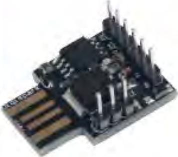
The Digispark Mini is a 26mm x 12mm sized microcontroller. It can be directly programmed via the Arduino IDE. It is also equipped with 6 I/O Pins, 8K Flash, I2C and SPI.
