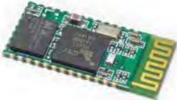
HC-05 module is an easy to use Bluetooth SPP (Serial Port Protocol) module, designed for transparent wireless serial connection setup.
