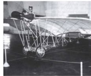
Santos-Dumont: First airplane built with bamboo, Paris 1907
