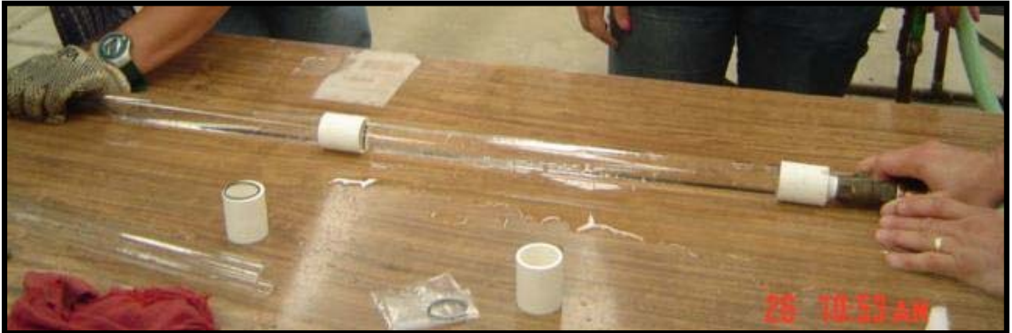
Figure 0-4. Visual inspection of PVC fittings between two glass tubes.
