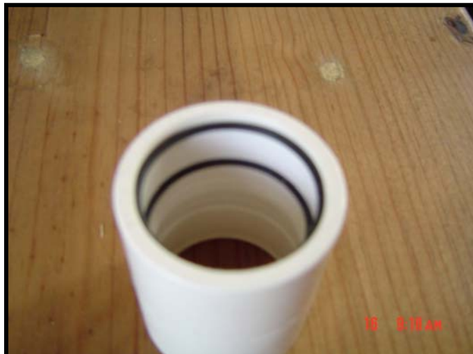
Figure 6-5 PVC coupling with two canals to fit O-rings
