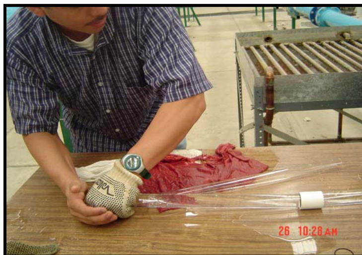
Figure O-3. Hand holding of the end of the tube to maintain pressure in the system.
