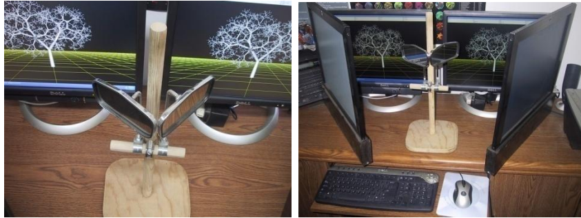
Figure 5.7 : 1) Placement of the small mirrors. 2) The Cazes-type digital stereoscope.
