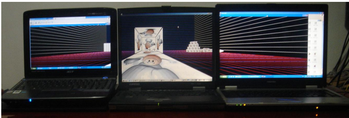
Figure 3.29 Three coplanar monitors displaying a virtual world
