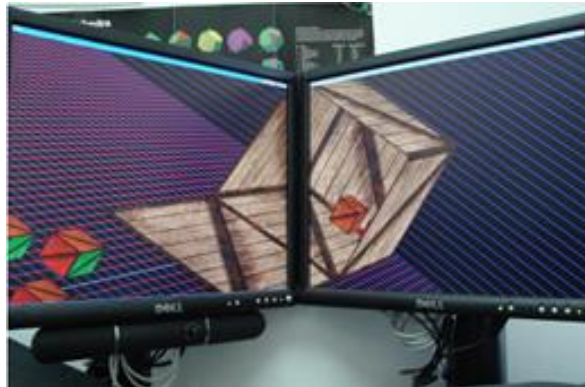
Figure 3.28 Two monitors forming a right angle and displaying a continuous and coherent image.
