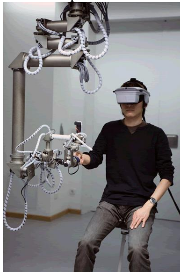
Figure 2.7 Haptic interaction with the hyper-redundant haptic display
