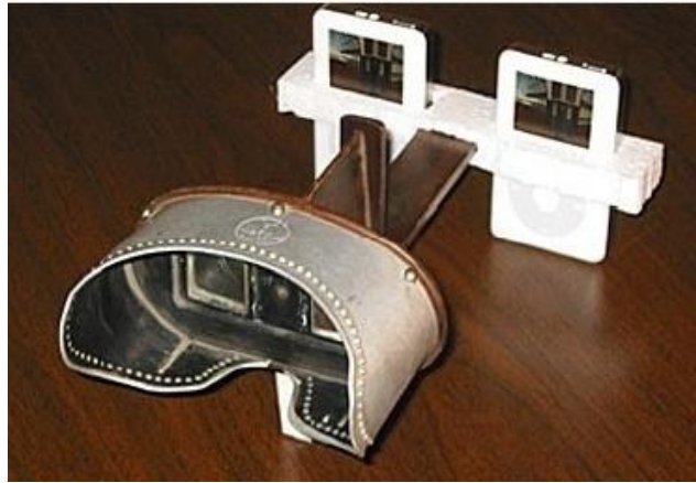
Figure 1.9 Holmes-type digital stereoscope built with two iPods
