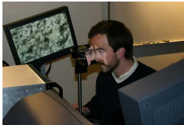
Figure 1.10 Wheatstone-type digital stereoscope built with two monitors
