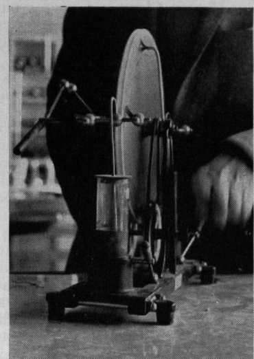
Familiar to most physics students is this "spark machine," located in the science department. The amber wheel rubbing against the brushes causes sparks to fly across the gap between the metal modules.
